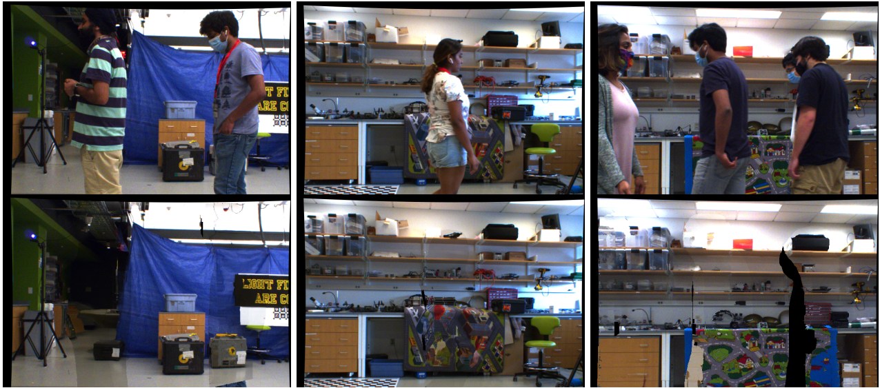
Fig. 5: Top row : Original images in the reference view. Bottom row : Refocused image of the static background. First column shows the result with some low textured regions. The second column shows the same in the presence of a lot of detail. Third column shows the case when dynamic objects dominate the scene.
